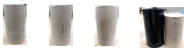
Failure patterns at different strain rates Behavior of GMC under several strain rates in confined loading condition (400 kPa confining pressure)
