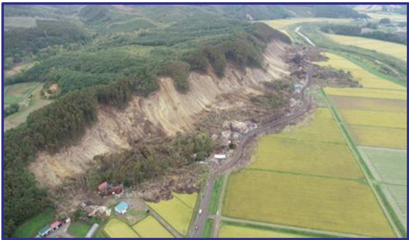
Slope failure after 2018 Hokkaido Eastern Iburi Earthquake
